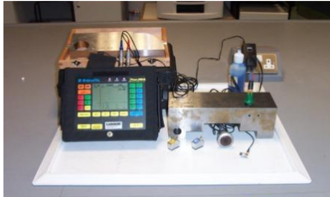
Ultrasonic Testing (UT) Equipment
