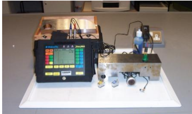
Ultrasonic Testing (UT) Equipment
