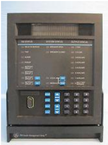
GE Multilin Relay 469 Simulator
