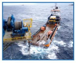
This course emphasizes the importance of good preparation for anchor handling, detailed knowledge of the job, continuous risk assessment and a methodical execution of each phase of the operations. These are the bases of a successful anchor handling operations.
